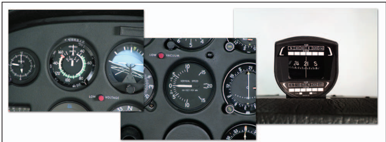
Figure 2-5. Airspeed indicator, VSI, and magnetic compass.
