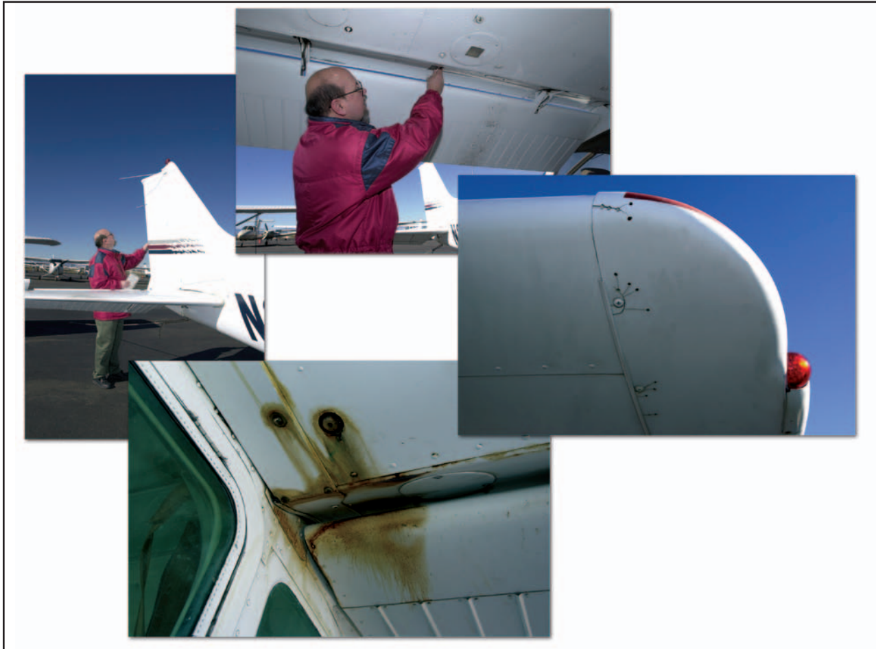
Figure 2-6. Wing and tail section inspection.
